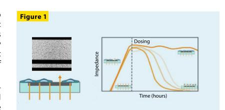
The impedance is measured from electrodes embedded in the **bottom of each well.** As cells cover more of the electrode. impedance increases in proportion to the number of attached cells. If a perturbation kills the attached cells, impedance decreases as the cells lyse.
